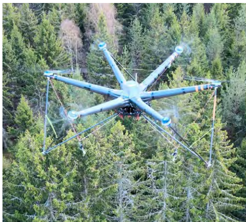
AirForestry is developing technology for thinning using drones.
